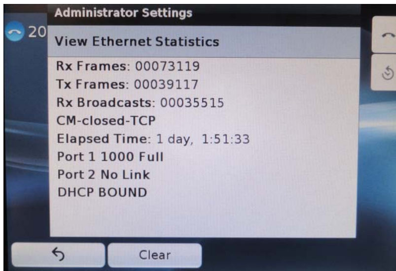
Figure 6-16 Cisco 9971 Phone Ethernet Statistics Screen
