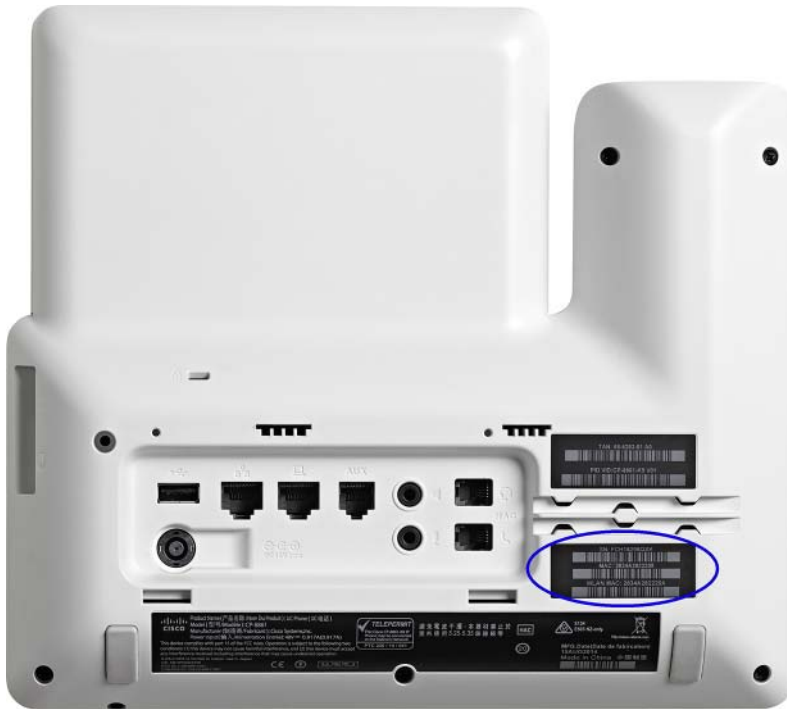
Figure 6-6 Cisco 8861 IP Phone MAC Address Location
