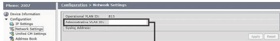
Figure 8-5 Static IP address and Administrative VLAN ID Configurations on CTS 500-32
