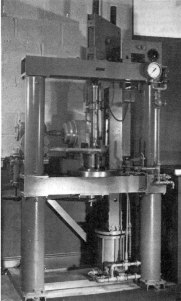
Figure 31 - Kneading Compactor and Diagram of Tamping Foot for Kneading Compactor. Reprinted with Permission of The Asphalt Institute
