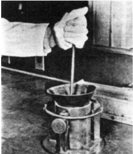
Figure 30 - Transferring the Mix to and rodding Mix in the Mold. Reprinted with Permission of The Asphalt Institute
