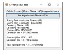
Fig. 21.3 | Fibonacci calculations performed in separate threads. (Part 3 of 3.)
