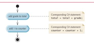
**Fig. 5.1** Sequence structure activity diagram.
