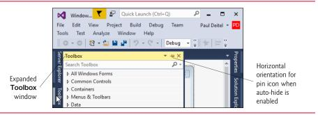
Fig. 2.11 | Displaying the hidden Toolbox window when auto-hide is enabled. www.hellodigi.ir
