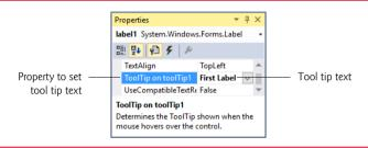
**Fig. 14.34** | Setting a control's tool tip text.
