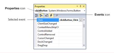
Fig. 14.8 Viewing events for a Button control in the Properties window.
