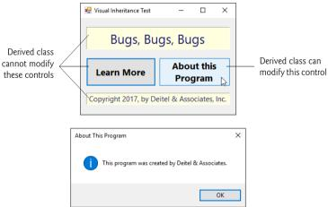
**Fig. 15.48** Derived Form using visual inheritance.
