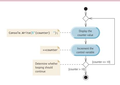
**Fig. 6.8** do...while iteration statement UML activity diagram.
