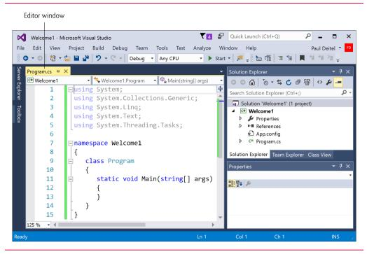
**Fig. 3.4** | IDE with an open console app's code displayed in the editor and the project's contents shown in the **Solution Explorer** at the IDE's top-right side.
