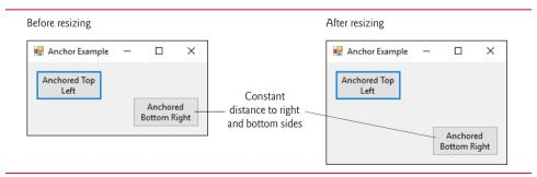
Fig. 14.13 Anchoring demonstration.
