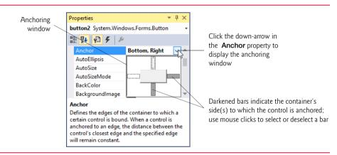
Fig. 14.12 Manipulating the **Anchor** property of a control.
