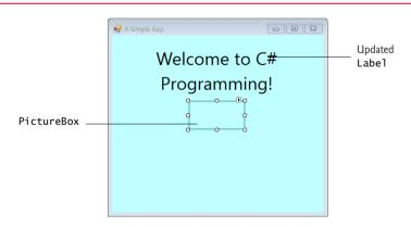
Fig. 2.29 | Inserting and aligning a PictureBox.
