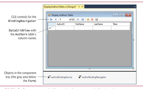
Fig. 20.21 Component tray holds nonvisual components in **Design** view.
