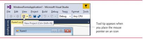
**Fig. 2.9** | Tool tip for the **New Project** button.
