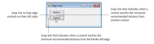
**Fig. 14.16** | Snap lines for aligning controls.
