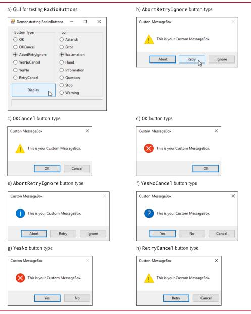
Fig. 14.28 | Using RadioButtons to set message-window options. (Part 4 of 4.)
