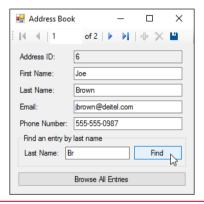
**Fig. 20.39** Type a search string in the **Last Name** TextBox, then press **Find** to locate contacts whose last names begin with that string. Only two names start with **Br**, so the **BindingNavigator** shows the first of two matching records.
