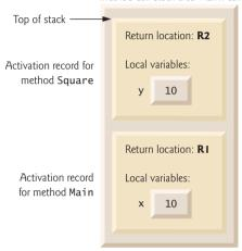
Fig. 7.11 Method-call stack after Main calls square to perform the calculation.
