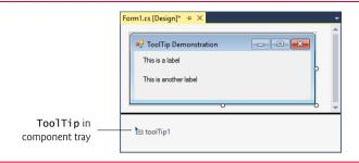
**Fig. 14.33** Demonstrating the component tray.
