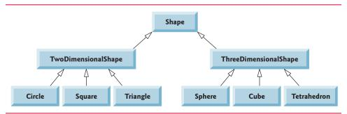
UML class diagram showing an inheritance hierarchy for Shapes. www.hellodigi.ir
