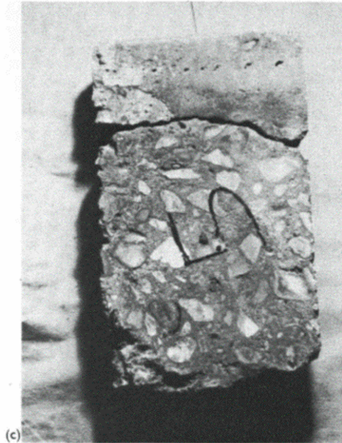
Fig. 5.16 Cores extracted in 1983 from a 1930s reinforced concrete factory building: (a) uncoated concrete from interior surface; (b) concrete coated in 1952; (c) core from an area repaired with mortar and coated in 1952. The cores have been sprayed with phenolphthalein solution; lighter areas indicate depth of carbonation. (Courtesy of W.J. Leigh & Co.)
