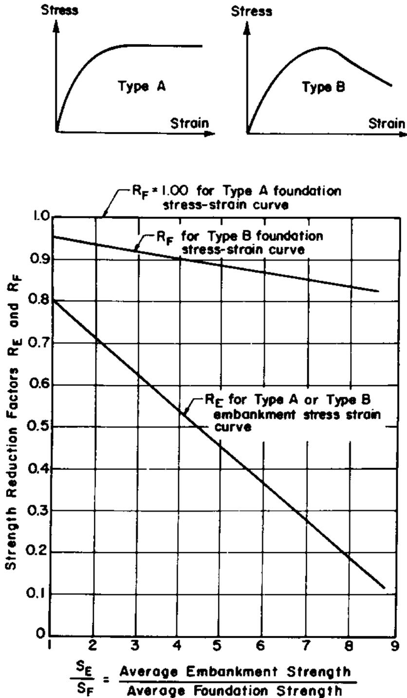
Figure 7-5. Peak strength correction factors for both embankment and foundation to prevent progressive failure in the foundation for embankments on soft clay foundations (Duncan and Buchignani 1975)
