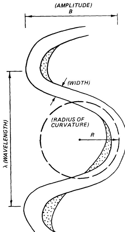
Figure 4-5. Meander geometry
