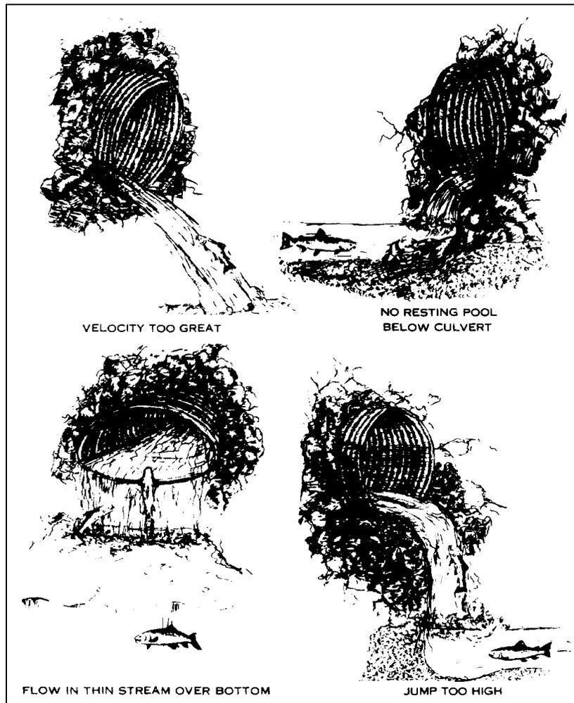
Figure 4-9. Culvert blockages to fish movement
