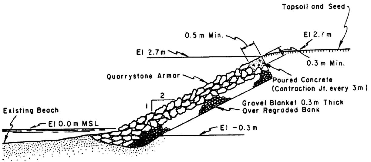
Figure 5-3. Quarrystone revetment
