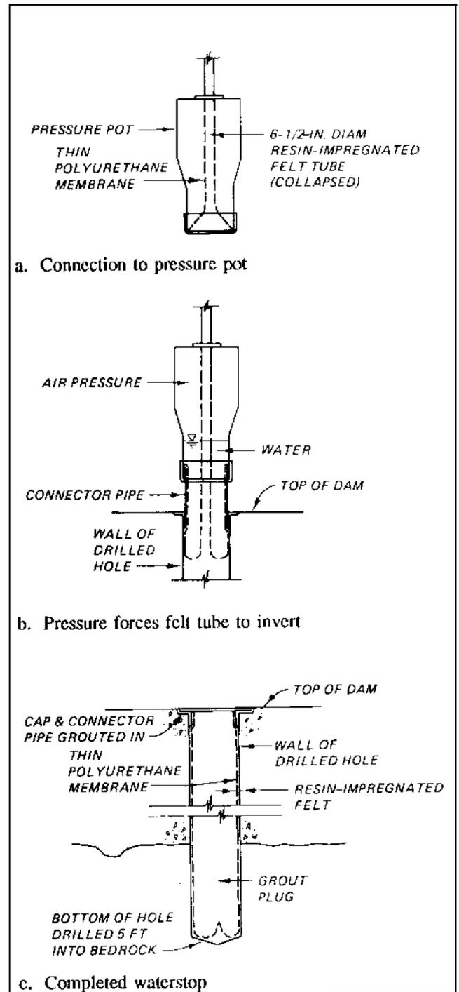
**Figure 8-25. Remedial waterstop installation, Pine Flat Dam**
