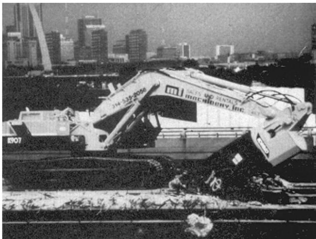
**Figure 5-2. Boom-mounted concrete crusher**
