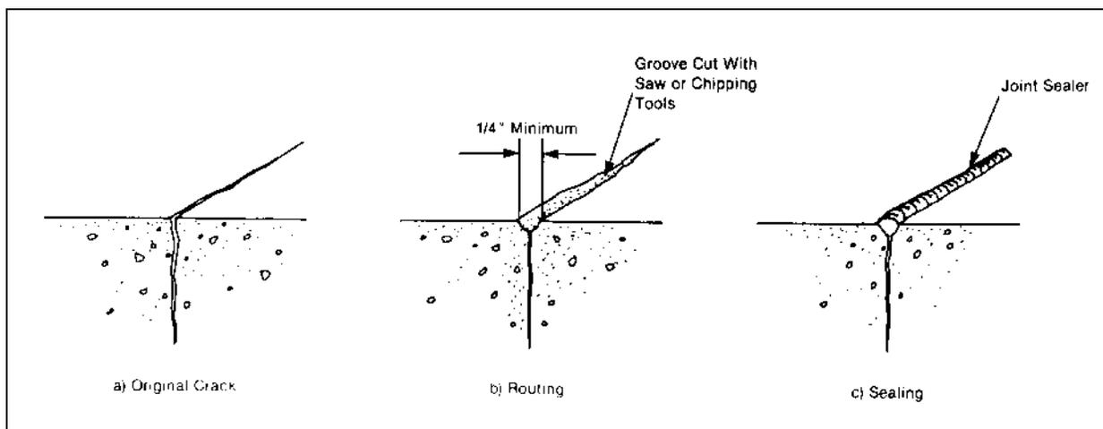
Figure 6-10. Repair of crack by routing and sealing
