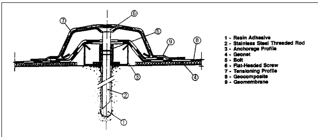
Figure 8-58. Detail of vertical anchorage and drainage profile
