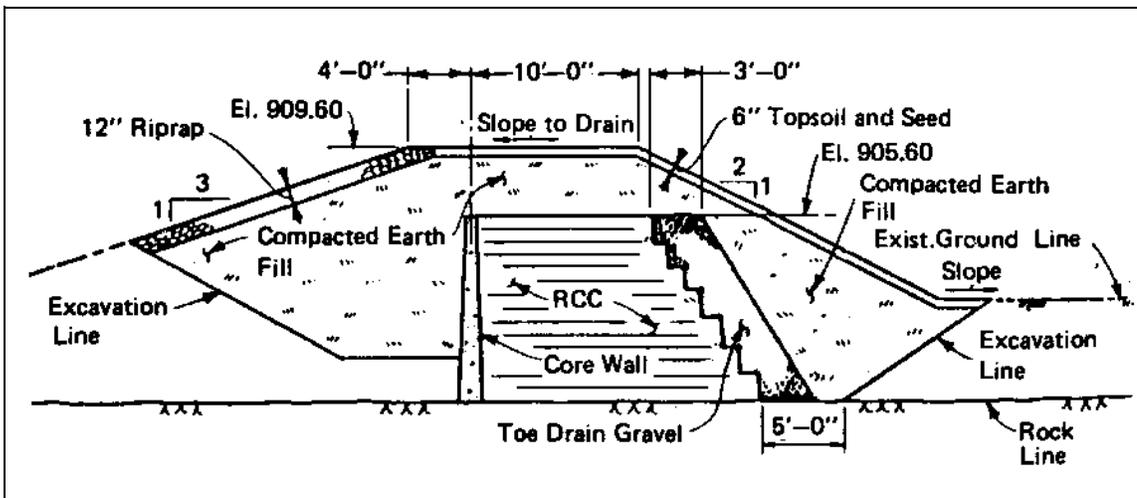
Figure 8-67. RCC spillway section, Boney Falls Dam (Marold 1992)
