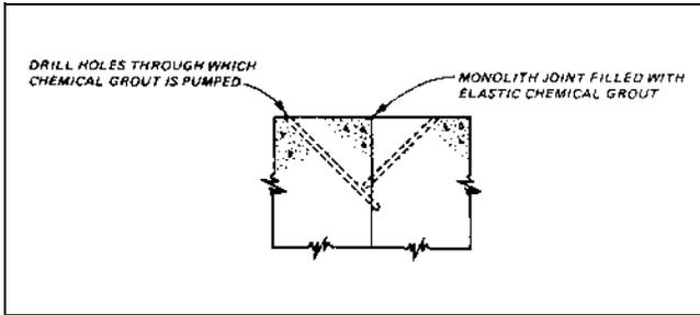
Figure 8-26. Joint filled with elastic grout through injection
