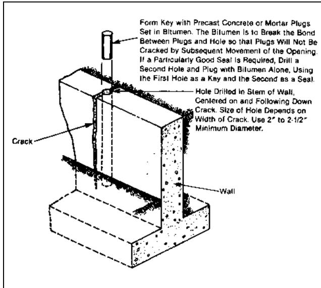
Figure 6-5. Repair of crack by drilling and plugging
