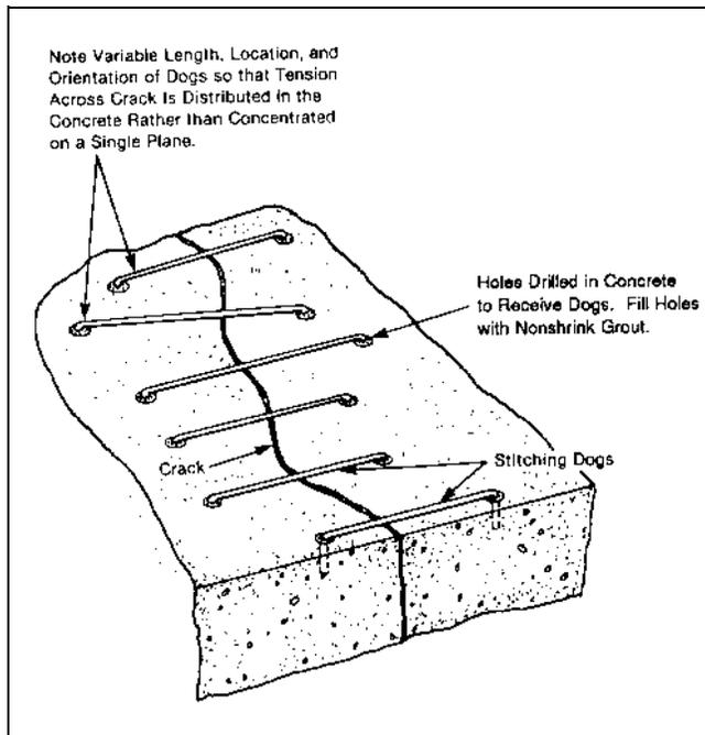
Figure 6-13. Repair of a crack by stitching
