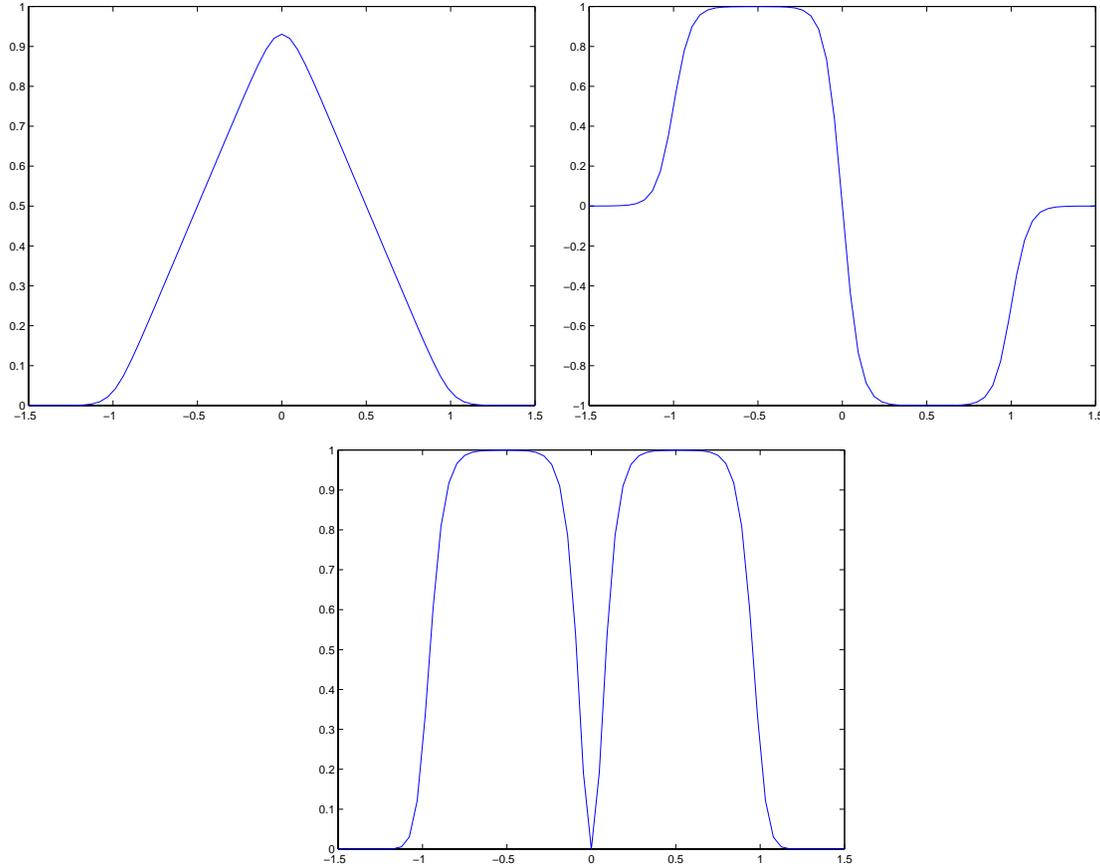
Figure 3.2.1: Smooth version of a piecewise linear hat function (3.2.7) (top), its first derivative (center), and the square of its first derivative (bottom). Results are shown with  $x_{j-1} = -1$ ,  $x_j = 0$ ,  $x_{j+1} = 1$  ( $h = 1$ ), and  $n = 10$ .
