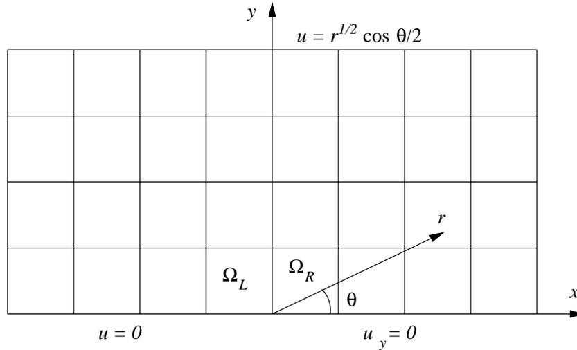
Figure 7.4.4: Cracked panel used for Example 7.4.4.
