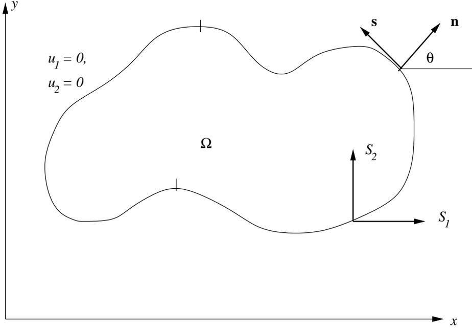
Figure 3.1.2: Two-dimensional elastic sheet occupying the region  $\Omega$ . Displacement components  $(u_1, u_2)$  vanish on  $\partial\Omega_E$  and traction components  $(S_1, S_2)$  are prescribed on  $\partial\Omega_N$ .
