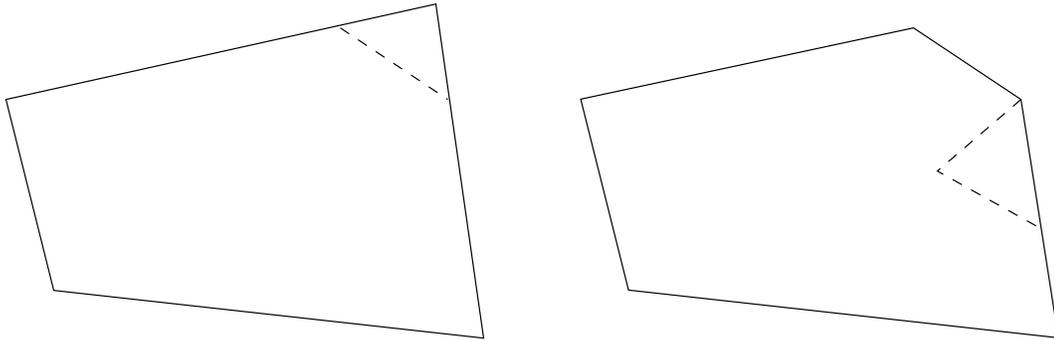
Figure 5.2.7: Mesh generation by the advancing front technique.
