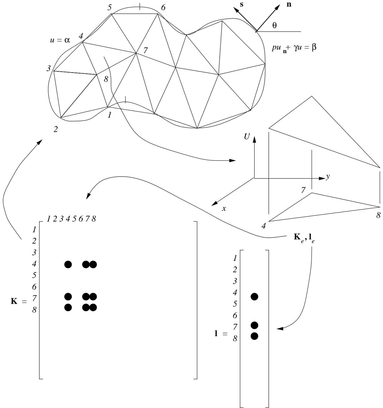
Figure 3.3.1: Two-dimensional domain  $\Omega$  having boundary  $\partial\Omega = \partial\Omega_E \cup \partial\Omega_N$  with unit normal  $\mathbf{n}$  discretized by triangular finite elements. Schematic representation of the assembly of the element stiffness matrix  $\mathbf{K}_e$  and element load vector  $\mathbf{l}_e$  into the global stiffness matrix  $\mathbf{K}$  and load vector  $\mathbf{l}$ .
