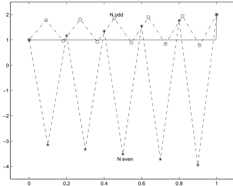
Figure 9.5.1: Solutions of (9.5.2) with  $\epsilon = 10^{-3}$ . The exact solution is shown as a solid line. Piecewise-linear Galerkin solutions with 10- and 11-element meshes are shown as dashed and dashed-dotted lines, respectively [1].
