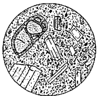
Microscope view, 5 mm across: clear feldspar laths, dark mafics, fine groundmass of same minerals.
