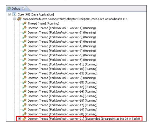
You can see that only the **worker-21** is suspended (marked in red in the screenshot) while the rest of the threads are running. However, if you change **Default suspend policy for new breakpoints** to **Suspend VM**, all the threads suspend their execution while you're debugging a concurrent application and the debug process hits a breakpoint. The following screenshot shows an example of this situation:
