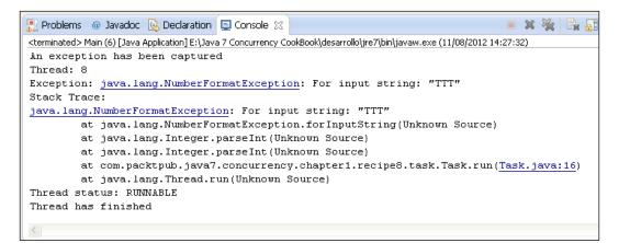
When an exception is thrown in a thread and is not caught (it has to be an unchecked exception), the JVM checks if the thread has an uncaught exception handler set by the corresponding method. If it has, the JVM invokes this method with the Thread object and Exception as arguments.
