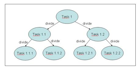
There is no formula to determine the reference size of a problem that determines if a task is subdivided or not, depending on its characteristics. You can use the number of elements to process in the task and an estimation of the execution time to determine the reference size. Test different reference sizes to choose the best one to your problem. You can consider ForkJoinPool as a special kind of Executor.
