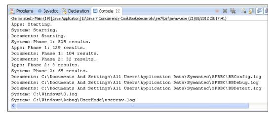
It shows the first two phases of the execution. You can see how the **Apps** thread finishes its execution in phase two because its results list is empty. When you execute the example, you will see how some threads finish a phase before the rest, but they wait until all have finished one phase before continuing with the rest.
