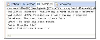
The example has two UserValidator objects that return a random boolean value. Each UserValidator object is used by a Callable object, implemented by the TaskValidator class. If the validate() method of the UserValidator class returns a false value, the TaskValidator class throws Exception. Otherwise, it returns the true value.
