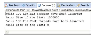
First, you have executed 100 AddTask tasks to add elements to the list. Each one of those tasks inserts 10,000 elements to the list using the add() method. This method adds the new elements at the end of the list. When all those tasks have finished, you have written in the console the number of elements of the list. At this moment, the list has 1,000,000 elements.
