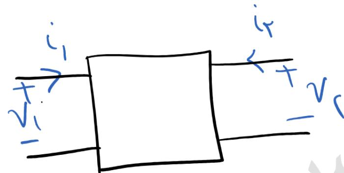
$$\begin{bmatrix} V_1 \\ V_{12} \end{bmatrix} = \underbrace{\begin{bmatrix} z_{11} & z_{12} \\ z_{21} & z_{22} \end{bmatrix}}_Z \begin{bmatrix} i_1 \\ i_2 \end{bmatrix}$$
